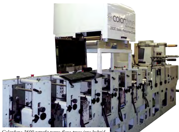
Colordyne 3600 retrofit turns flexo press into hybrid
