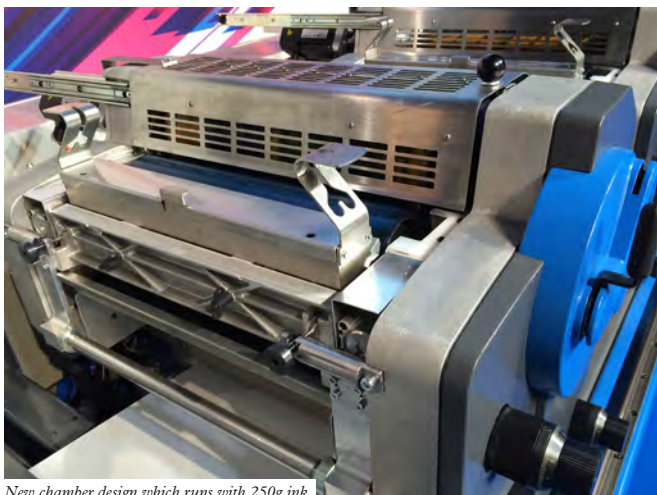
New chamber design which runs with 250g ink
