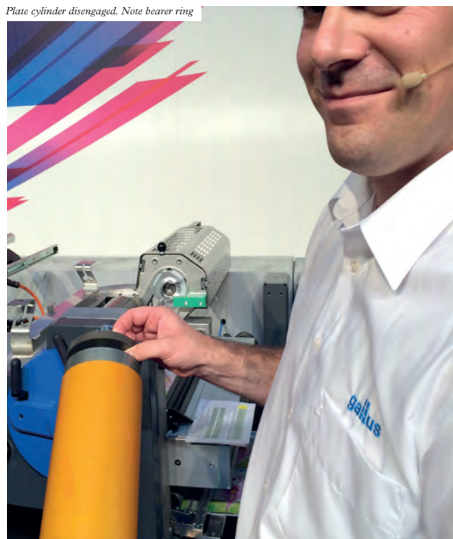
Plate cylinder disengaged. Note bearer ring
