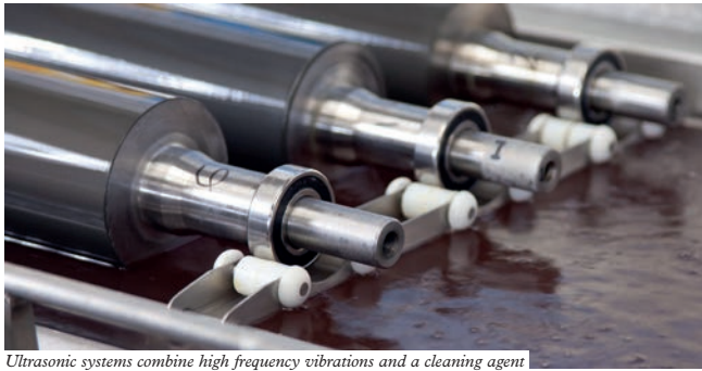
Ultrasonic systems combine high frequency vibrations and a cleaning agent
