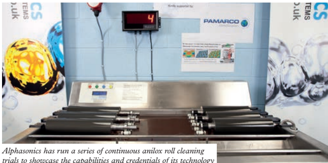
Ultrasonic systems combine high frequency vibrations and a cleaning agent
