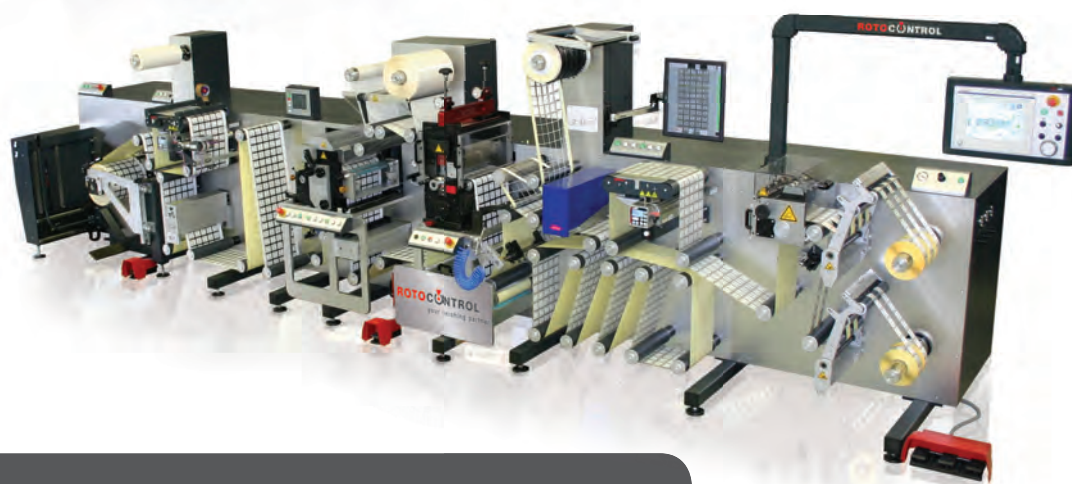
DT Series: For finishing digitally created labels
