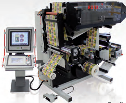
RSP Series: 100% inspection of pharmaceutical labels
