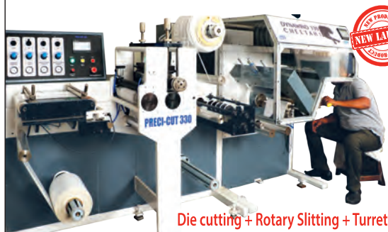
Servo slitting machine with 100% inspection
