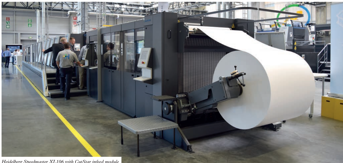
Heidelberg Speedmaster XL106 with CutStar infeed module
