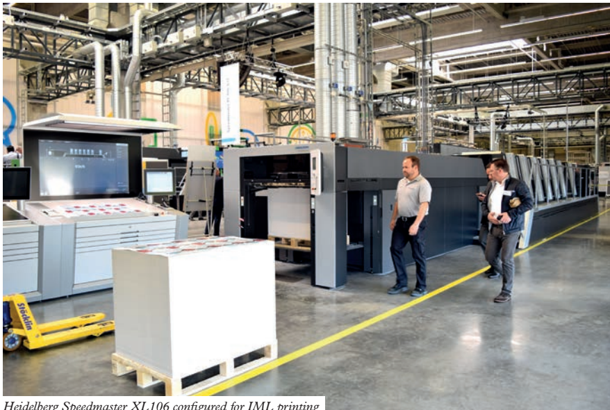
Heidelberg Speedmaster XL106 configured for IML printing
