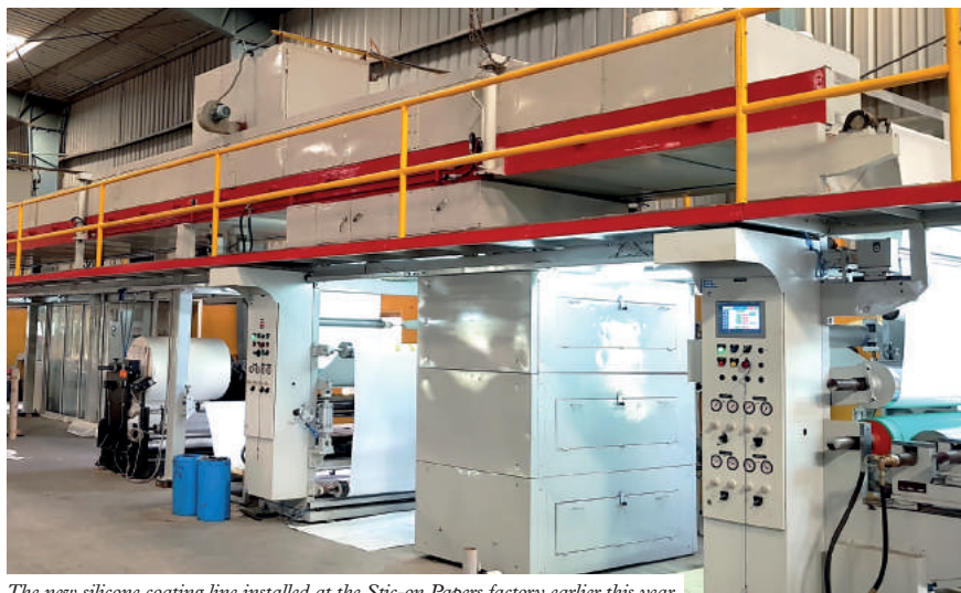
The new silicone coating line installed at the Stic-on Papers factory earlier this year
