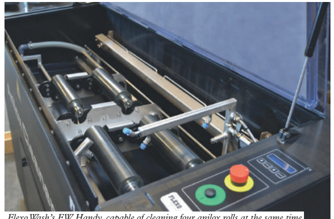
Flexo Wash's FW Handy, capable of cleaning four anilox rolls at the same time
