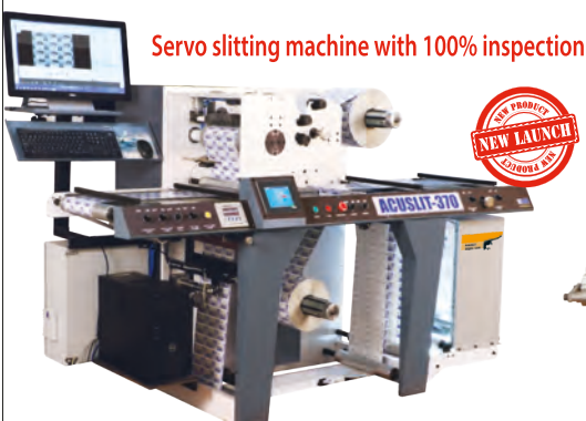
Die cutting + Rotary Slitting + Turret rewinder
