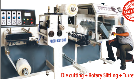
Servo slitting machine with 100% inspection
