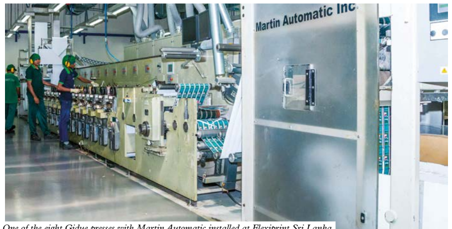
One of the eight Gidue presses with Martin Automatic installed at Flexiprint Sri Lanka
