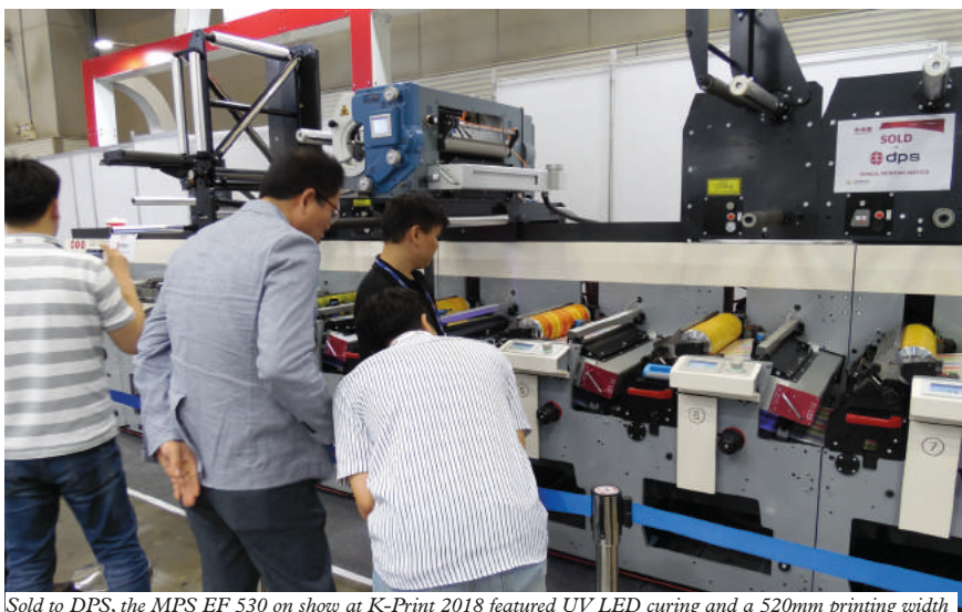
Sold to DPS, the MPS EF 530 on show at K-Print 2018 featured UV LED curing and a 520mm printing width
