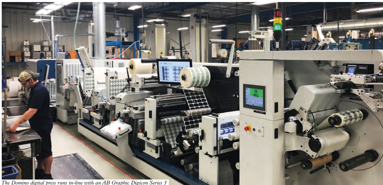
The Domino digital press runs in-line with an AB Graphic Digicon Series 3
