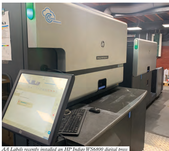
AA Labels recently installed an HP Indigo WS6800 digital press
