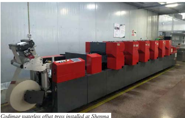
Codimag waterless offset press installed at Shenma
