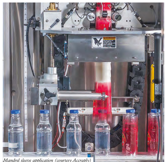
Mandrel sleeve application (courtesy Accraply)
