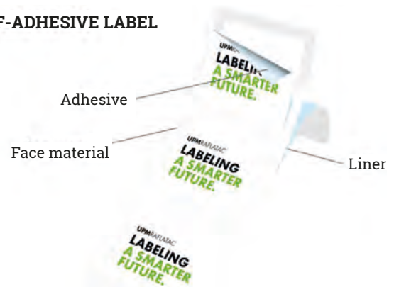
Composition of self-adhesive roll (courtesy UPM Raflatac)
