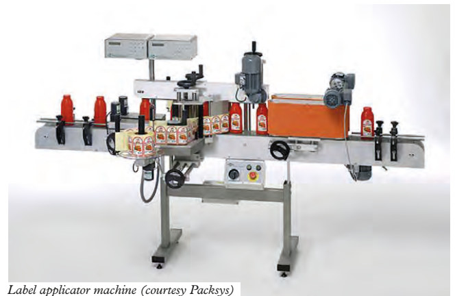
Label applicator machine (courtesy Packsys)
