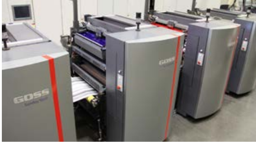
Precision Press has been 'extremely pleased' with its Sunday Vpak 500 model, including in-line flexo coating unit, along with UV and EB curing capabilities
