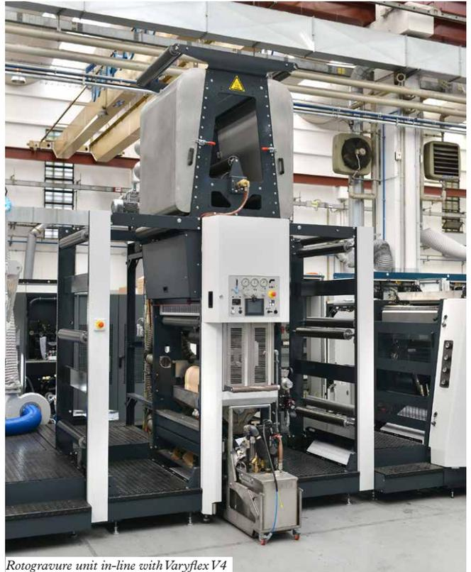
Rotogravure unit in-line with Varyflex V4
