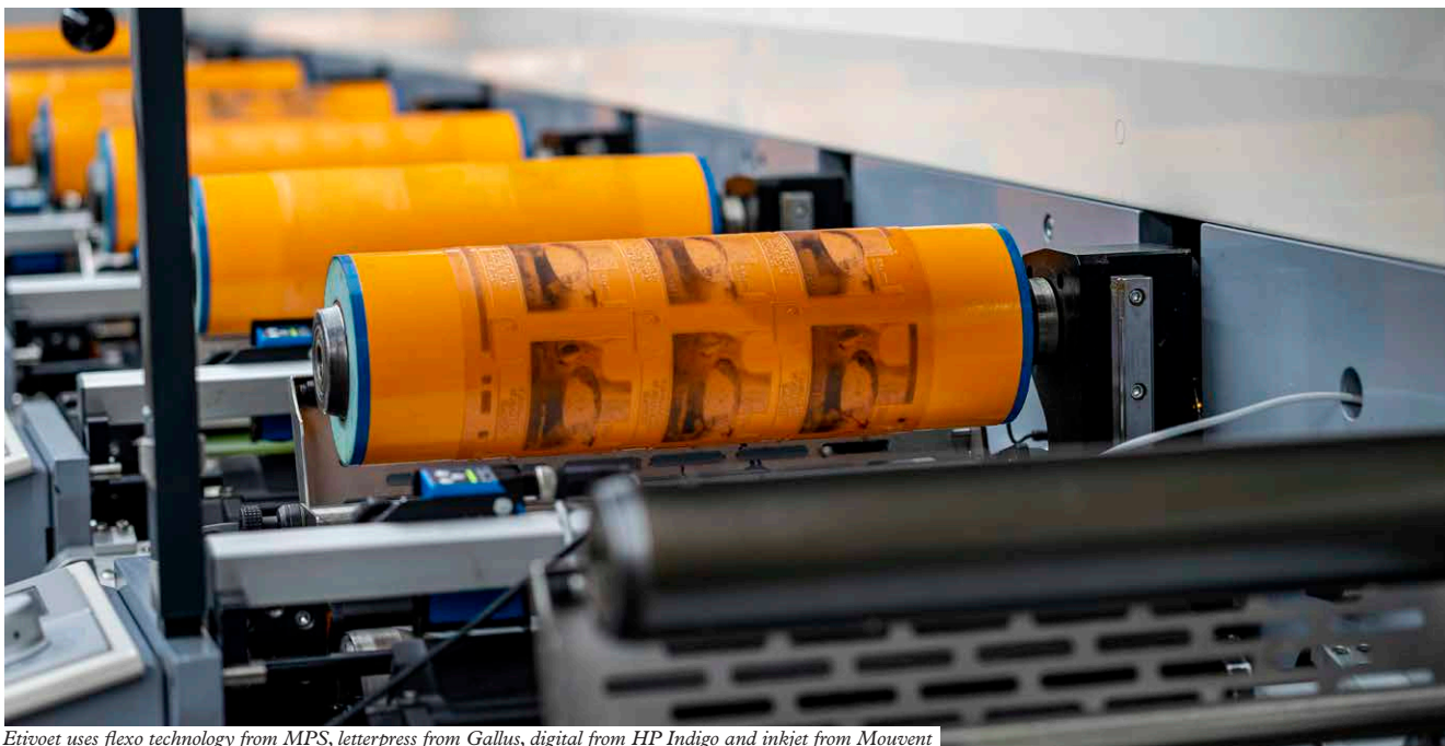
Etivoeet uses flexo technology from MPS, letterpress from Gallus, digital from HP Indigo and inkjet from Mouvent
