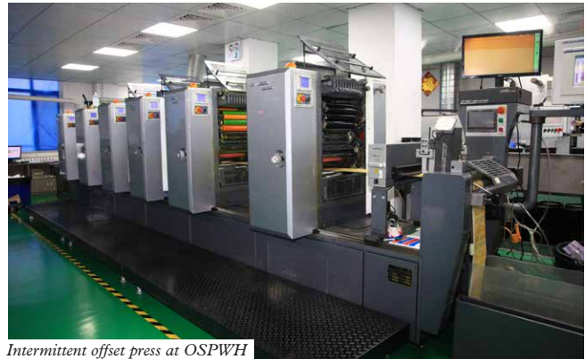
Intermittent offset press at OSPWH
