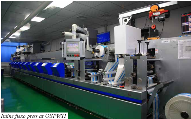
Inline flexo press at OSPWH
