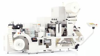
Prati highlights DigiCompact, a converting and finishing line for self-adhesive labels and digitally printed flexible packaging
