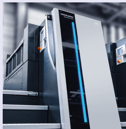
XL106 coating unit with AutoPlate Coating Pro automation
