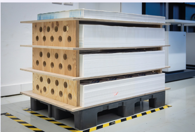
The hurdle delivery improves pile formation when printing on IML films and similar substrates
