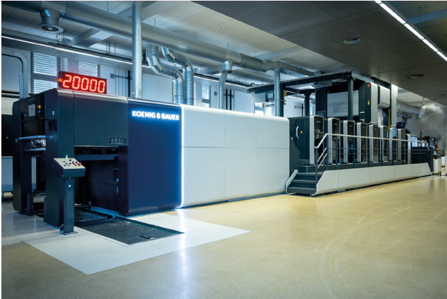
Rapida 106 X in a typical configuration for label production - seven printing units, RS 106 X reel-to-sheet feeder, cold foil module, in-line coater with AniloxLoader and extended delivery
