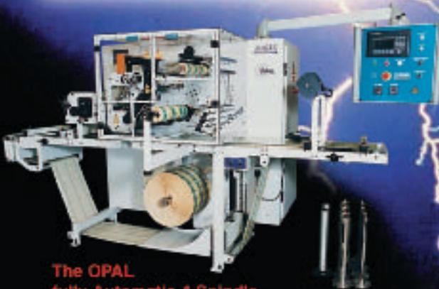
The OPAL fully Automatic 4 Spindle Turret Model, comes in a choice of three working widths, 330, 410 or 510 mm.
