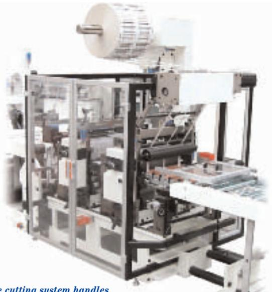
Omet Twin Cut die cutting system handles multiple repeats without cylinder change
