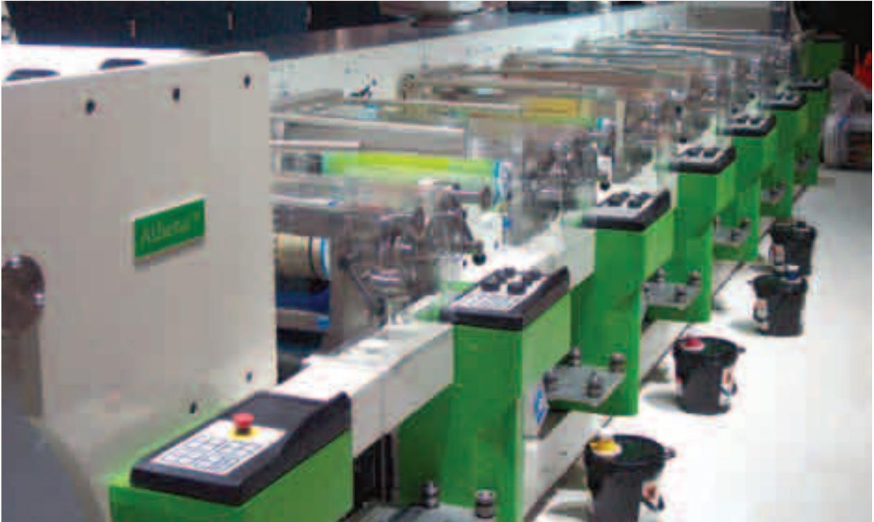
*The GiDue Athena mid-web flexo press. Note the arrangement of the anilox roll beneath the plate cylinder*
