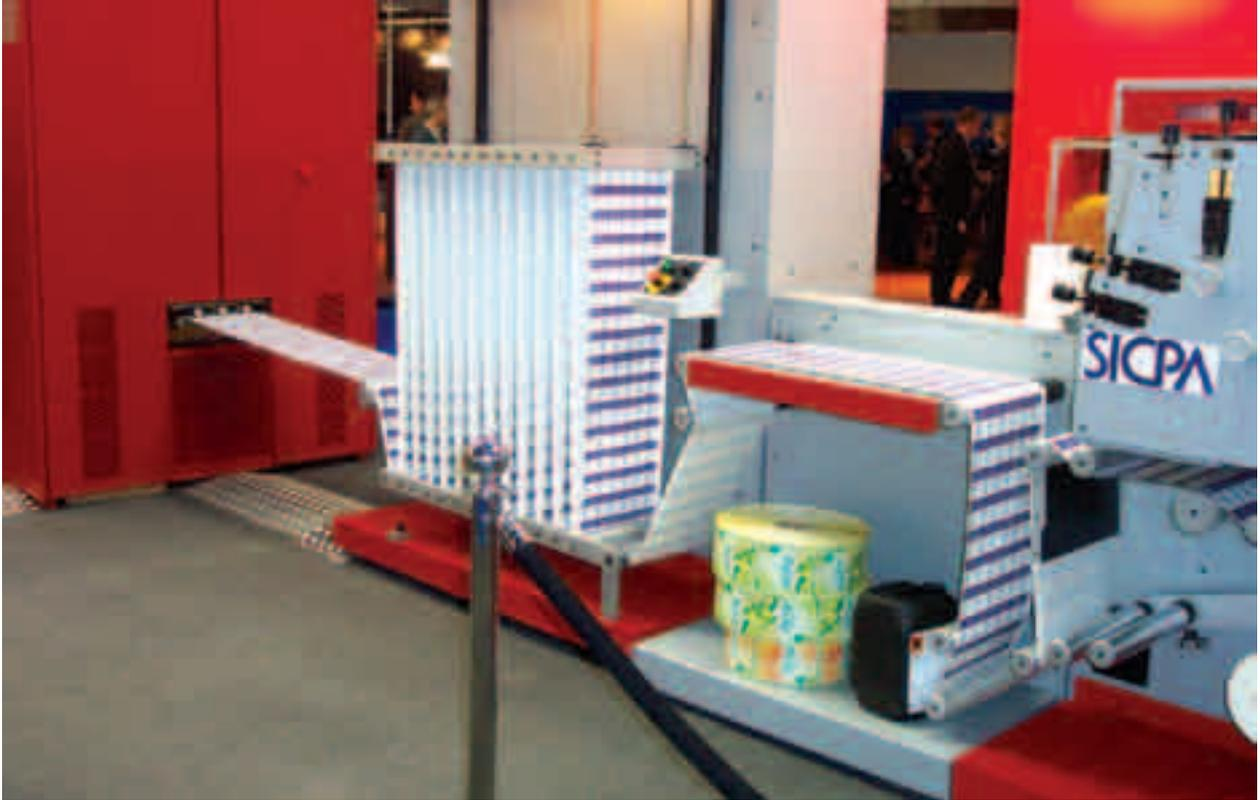
*The LabelSprint digital press from Xeikon with in-line D-coat finishing*
