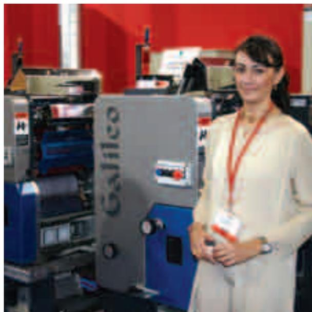
(Left) Print unit of the Muller Martini variable-size Alprinta-V press. (Above) The Franchini Galileo offset combination press
