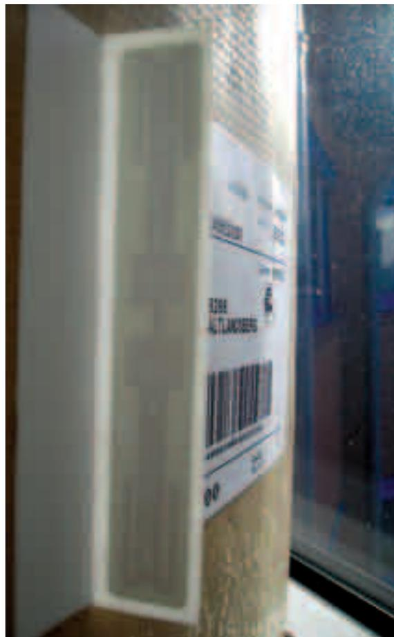
*Testing of the RFID system under realistic conditions was essential, as in practice the range which can be achieved is extremely sensitive to variations in the type of packaging and the contents within*
