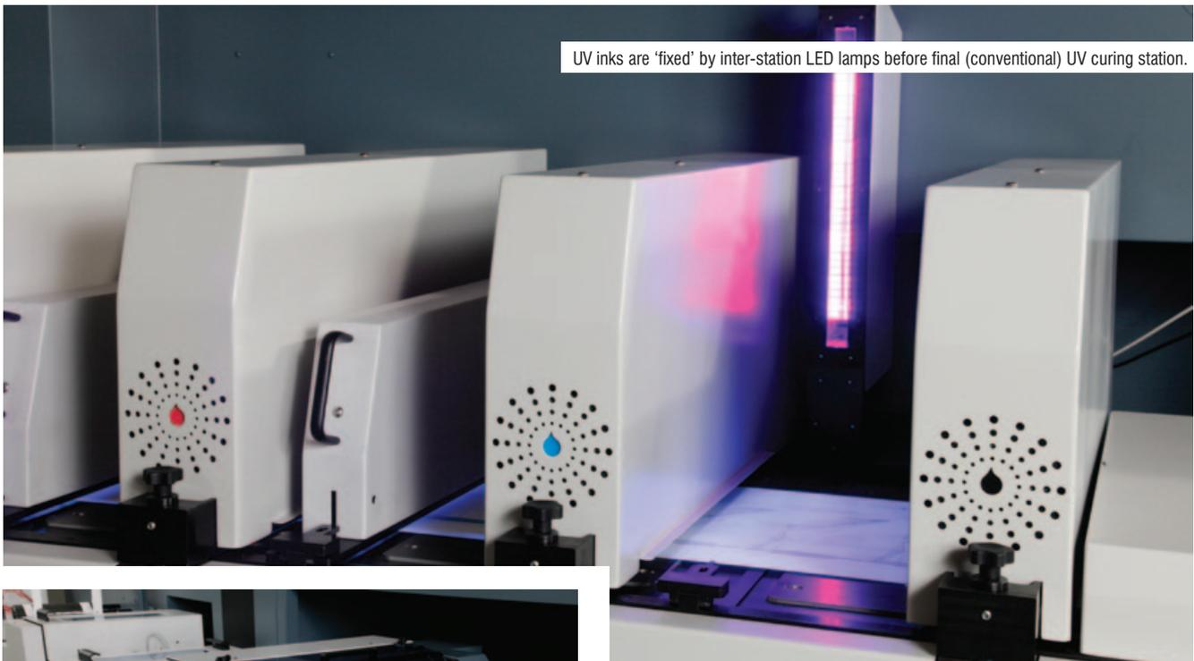
UV inks are 'fixed' by inter-station LED lamps before final (conventional) UV curing station.
