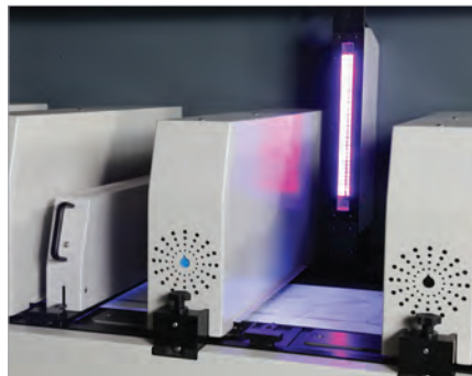
UV LED pinning for supporting optimal text and line definition
