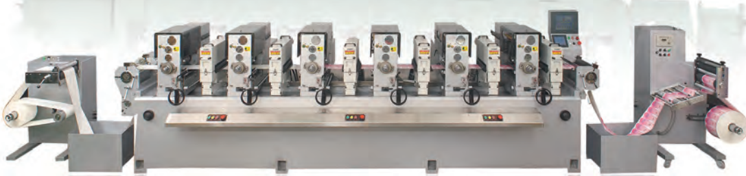
FD-300 Intermittent Letterpress Label Printing Machine
