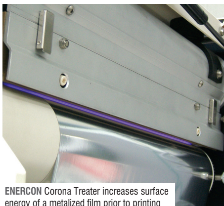
FIG. 1 An example of the effects of corona treatment and ink adhesion
