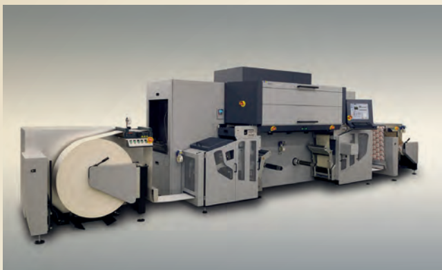
New options for Durst's Tau 330 digital label press include an industrial scale jumbo roll unwinder/rewinder
