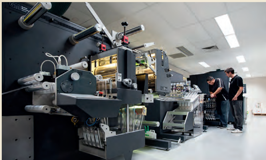
GM's established 'mini' series of in-line converting systems for digital presses has been upgraded with cold foil/super gloss capability
