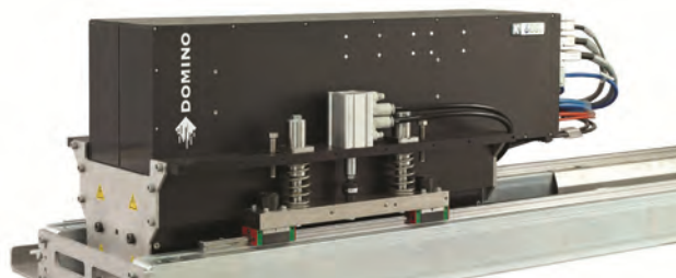
Domino shows its K600i digital UV inkjet printer integrated with an AB Graphic Omega SRI
