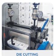
Rotary/semi-rotary die cutting with adjustable gap
