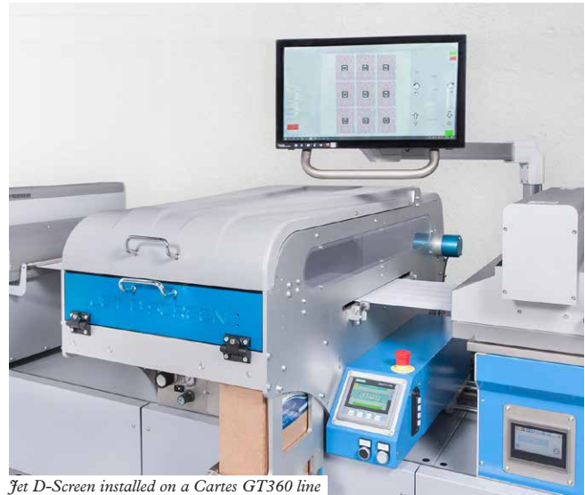
Jet D-Screen installed on a Cartes GT360 line
