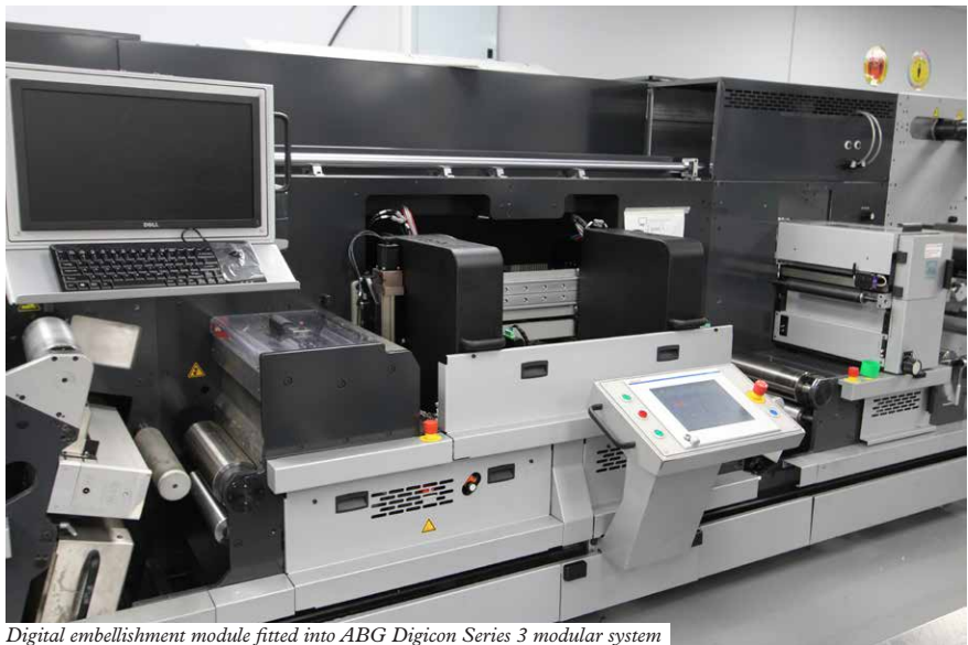
Digital embellishment module fitted into ABG Digicon Series 3 modular system
