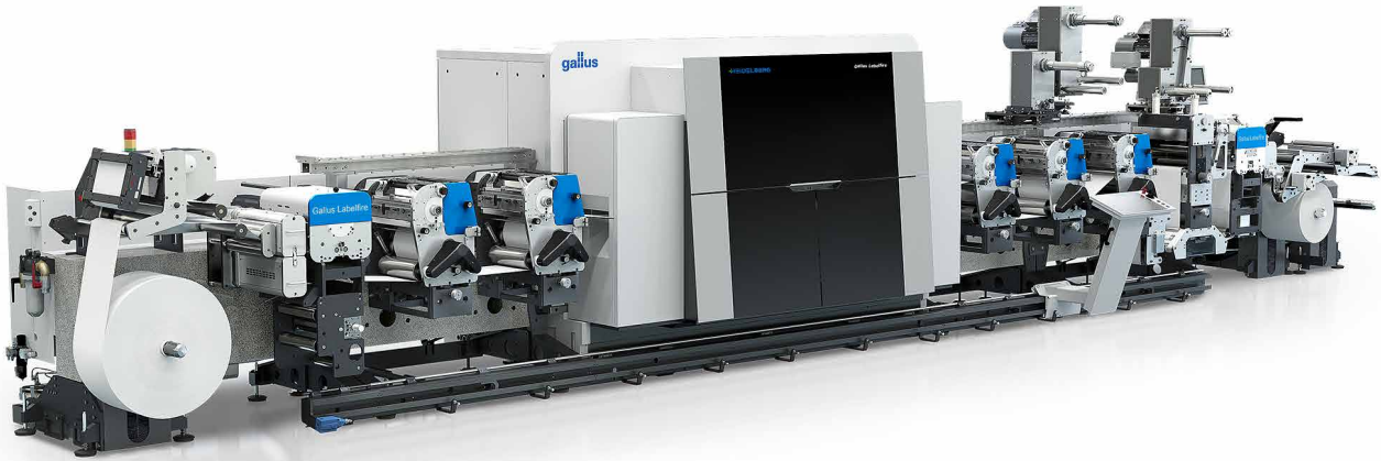
The next step for Labelfire will be both a wider 430mm web and a 250mm 4-color model
